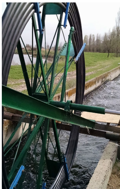
Above: This waterwheel pump was installed in a Central Asian aqueduct to give farmers access to water.
